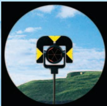
**Gone are the days when you had to spend a lot of time aiming at the target to be measured. Today, TPS700ultra and TPS700power total stations perform this task with automatic target recognition (ATR).**
