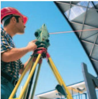
Gone are the days when hard to access targets could only be determined with a lot of effort. The PinPoint technology enables a reflectorless distance measurement to any surface at an exceptional range of over 500m ("TPS700ultra").
